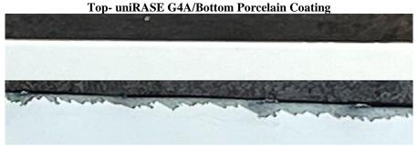
Conclusion- The uniRase G4A shows no to little edge flake, while the porcelain substrate fails and will require signifivant edge Repair.
