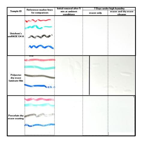
**Conclusion:** After 7-days of humidity exposure, the uniRASE G4A shows equal eraseability versus Porcelain and superior eraseability to the laminated film product. Additionally the laminated film shows poor hydrolitic stability, with signs of delamination, being apparent.
