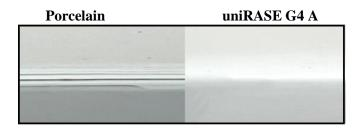
**Edge Flaking:** The coated metal substrate is cut using a metal shear. The brittleness of the coatings are evaluated. (NOTE: Polyester film was not included in this study, as the coating base, will dictate the performance.)
